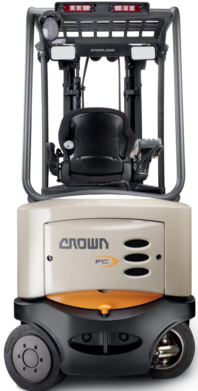
**Steer axle geometry** is engineered to minimize turning radius while extending steer tire life substantially beyond that of conventional trucks. Crown applies the correct turn angle in the FC 5200 Series to decrease tire wear over time.
