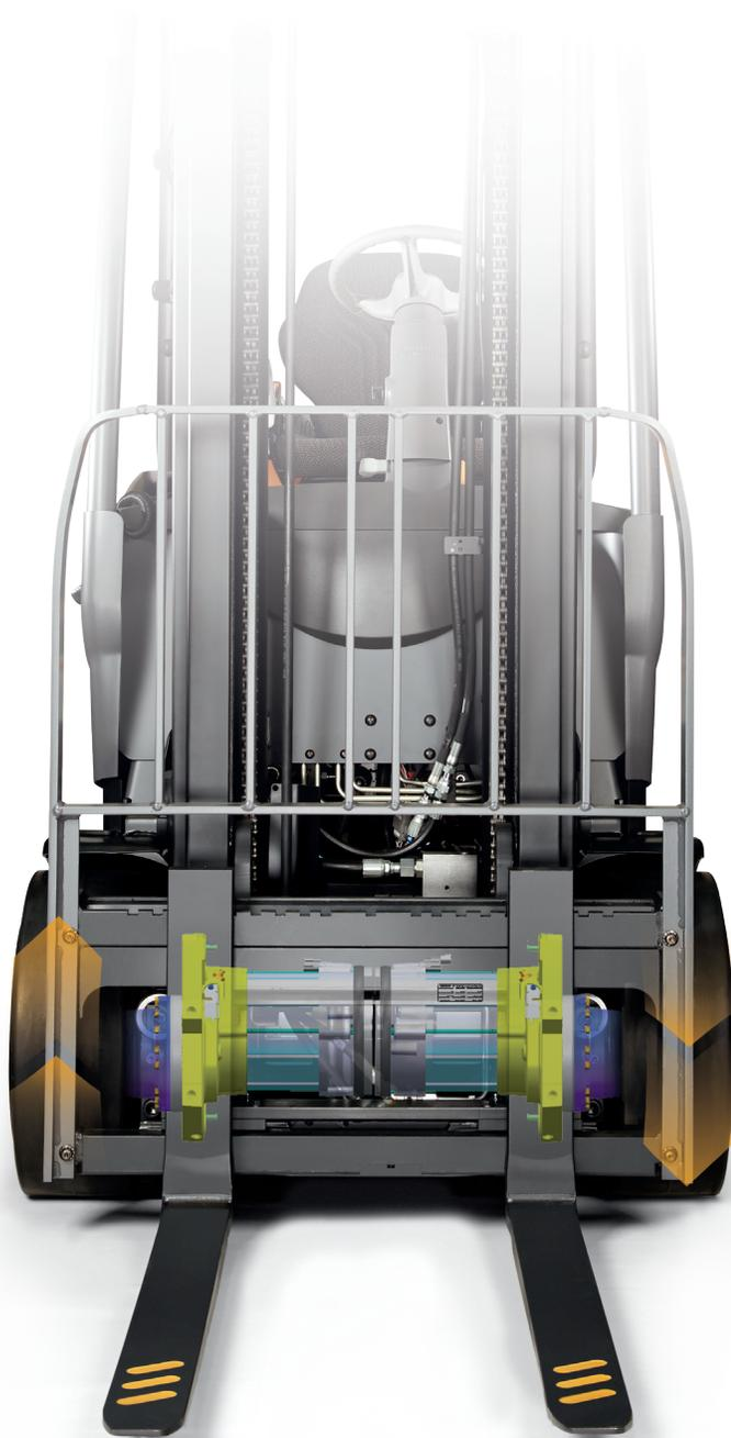
**Precise control** lets you take advantage of tighter right angle stacks. Larger, less maneuverable lift trucks require wider aisles, but drive motors turning in opposite directions allow the FC 5200 Series to spin 360 degrees in an aisle without disturbing surrounding pallets.
