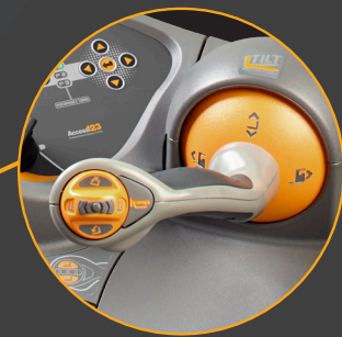
Multi-task Control Handle – features a comfortable grip and allows operators to blend functions.
