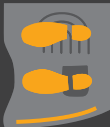
Brake and Presence Pedal – promotes safe operation with a dual-pedal design that discourages operators from using only one foot to operate the truck. Protects both the truck and the operator by automatically applying the brake when the operator's left foot is removed from the brake pedal. The roomier cabin and ability to adjust the position of the feet provide postural relief during travel.
