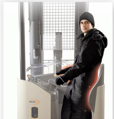
**ThermoAssist™ Package** offers a practical, cost-effective way to improve operator comfort and productivity. A mast air deflector and heated armrest and backpad (heated seat for S Class trucks) make cold environments more comfortable.
