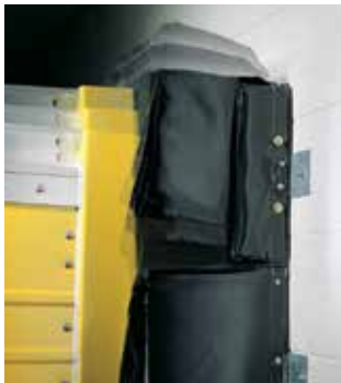
4" exposure wear pleating moves with the trailer, extending the life of the fabric in key wear areas.
