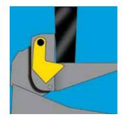
The Serco system's primary locking position provides a captive reach up to 11" to engage wide, recessed or bent rear impact guards and limits trailer movement.
