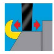
Rotating Hook systems feature a single-position lock that rotates to a horizontal position. Typical engagement can allow up to 7" of trailer movement with a standard rear impact guard.
